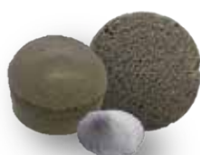
Silica fume geopolymer foams
