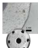
Wicks in Loop Heat Pipe (PON Project «PANDION»)
