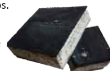
Porous cores and sandwich panels from industrial wastes and by-products (POR-FESR «EEE-CFCC»)
